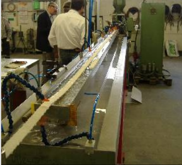
Rough strip from primary extruder
